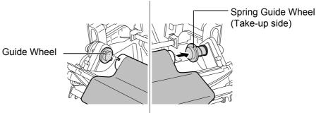
**5.** Turn the Ribbon Rewind Gear to wind the ribbon leading film onto the Ribbon Take-up Core until the ink ribbon covers the Print Head, and remove any slack of the ribbon.
